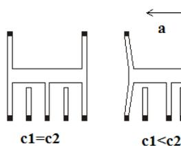
Figure 6 Operation of the acceleration sensor chip
