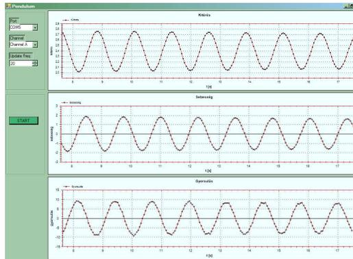
**Figure 10** The curves show the angular position, velocity and acceleration (from top to bottom, respectively)
