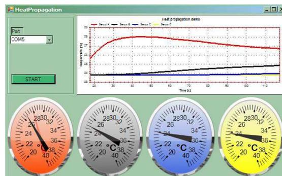
**Figure 3 The four curves correspond to the temperatures at the four equidistant points**
