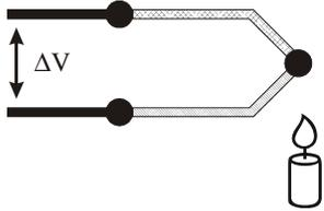
Figure 4 Construction of a typical thermocouple
