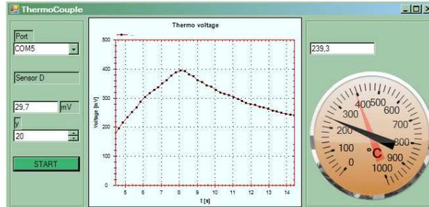
Figure 5 The curve shows the thermo voltage, the manometer shows the temperature (momentary and maximum)
