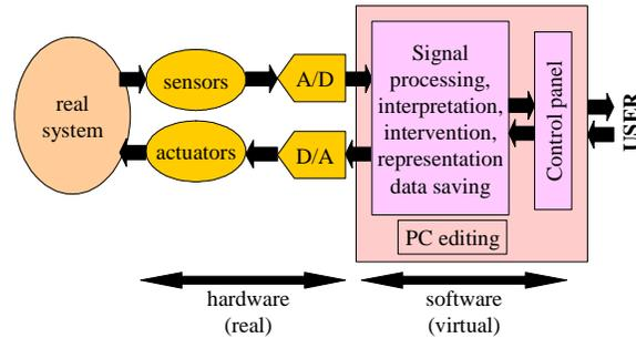
**Figure 1 System of a virtual instrument**
