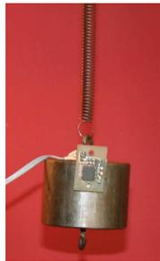
Figure 7 Combination of an acceleration sensor chip and a body hanging on a spring
