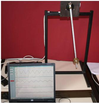
**Figure 9** Combination of a pendulum with a coaxial rotary potentiometer.
