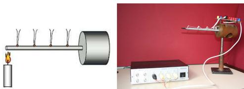
**Figure 2 Set a metal rod in a high-mass metal bulk and some thermistors equidistantly along the rod**
