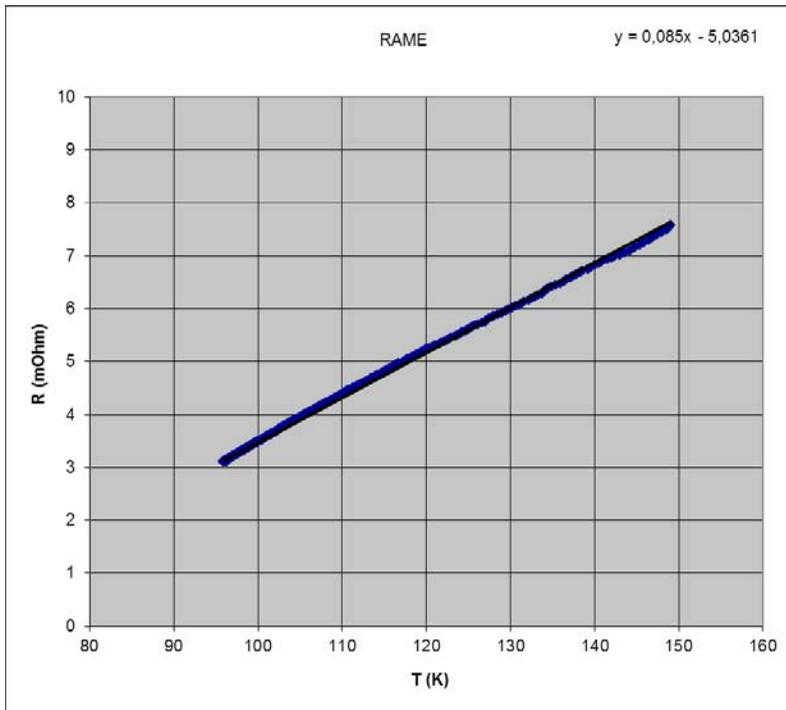
Figure 2. Copper resistance versus temperature
