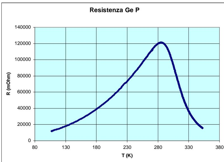
Figure 3. Ge::P resistance versus temperature
