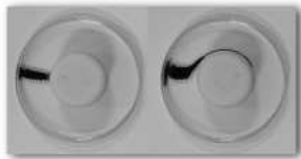
Figure 4: A cylinder is rotated while partly submerged in a thin layer of glycerine. A strip of black ink makes clear the no-slip condition close to the
