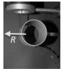
Figure 5: Coanda effect of water on a solid
