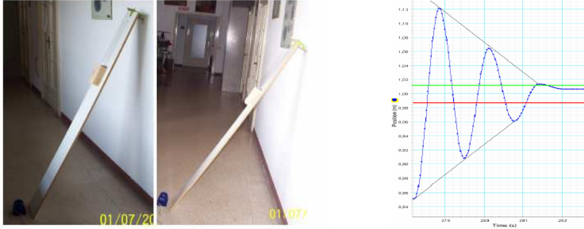
Figure 4: The experimental set up involving a periodic damped motion consists of a block-spring system placed on a wooden-inclined plane and a computer motion sensor at the bottom. Beneath the block four small plates of plastic material are placed.
