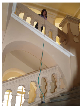
Figure 5: Underpressure 37100 Pa generated by lips (corresponds to 3,71m approx.)
